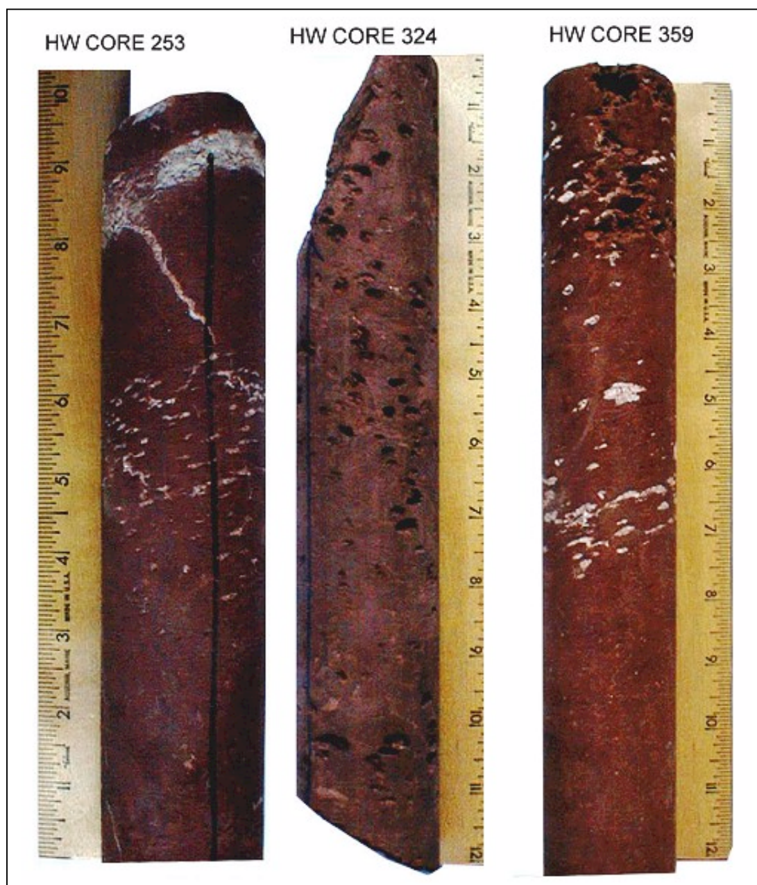
Figure 1.9. Examples of sparry minerals filling fractures and root cavity and other voids in HW 253 and 359 and dissolution-type-water bearing zones HW 324 and 359. Samples are from the HW core. Images from Herman (2001).
