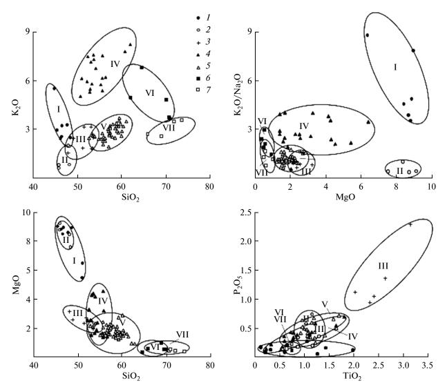
**Fig. 4.** Variation diagrams for melts of the Gorely volcanic center. Fields show the following melt types: (I) basic potassic melt; (II) basic sodic melt; (III) basic melt with high P and Ti concentrations; (IV) intermediate potassic melt; (V) intermediate sodic melt; (VI) acid potassic melt; (VII) acid sodic melt.
